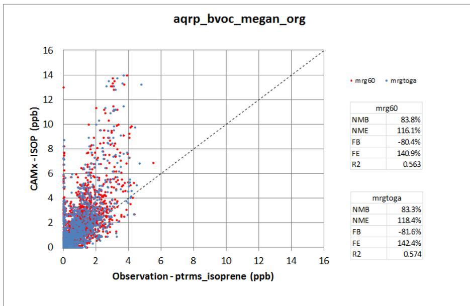
**Figure 2:** Comparison of CAMx modeled isoprene and isoprene measured by PTRMS along the C-130 flight tracks during the period June 1-July 14, 2013. mrg60 data are 1-minute averages of observed data, and mrgTOGA data are 2-minute averages.
